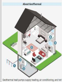
water for homes and buildings using the solar energy stored beneath the ground.
