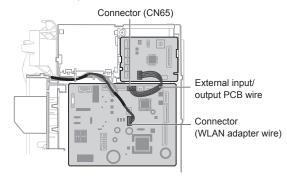
For the setting of rotary switch and DIP switch, refer to the installation manual of optional parts.
