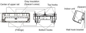
After hooking the indoor unit to the top hook, hook the fittings of the indoor unit to the bottom hooks while lowering the unit and pushing it against the wall
